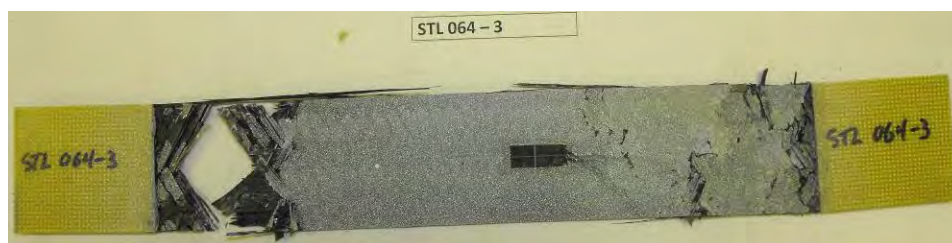
Figure 34. Strain Gage Location for Axial Modified ASTM D 3039 2D3A
