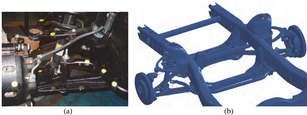
Figure 7.23. Steering stabilizer links: (a) actual model, (b) FE model (denoted by the red color).
