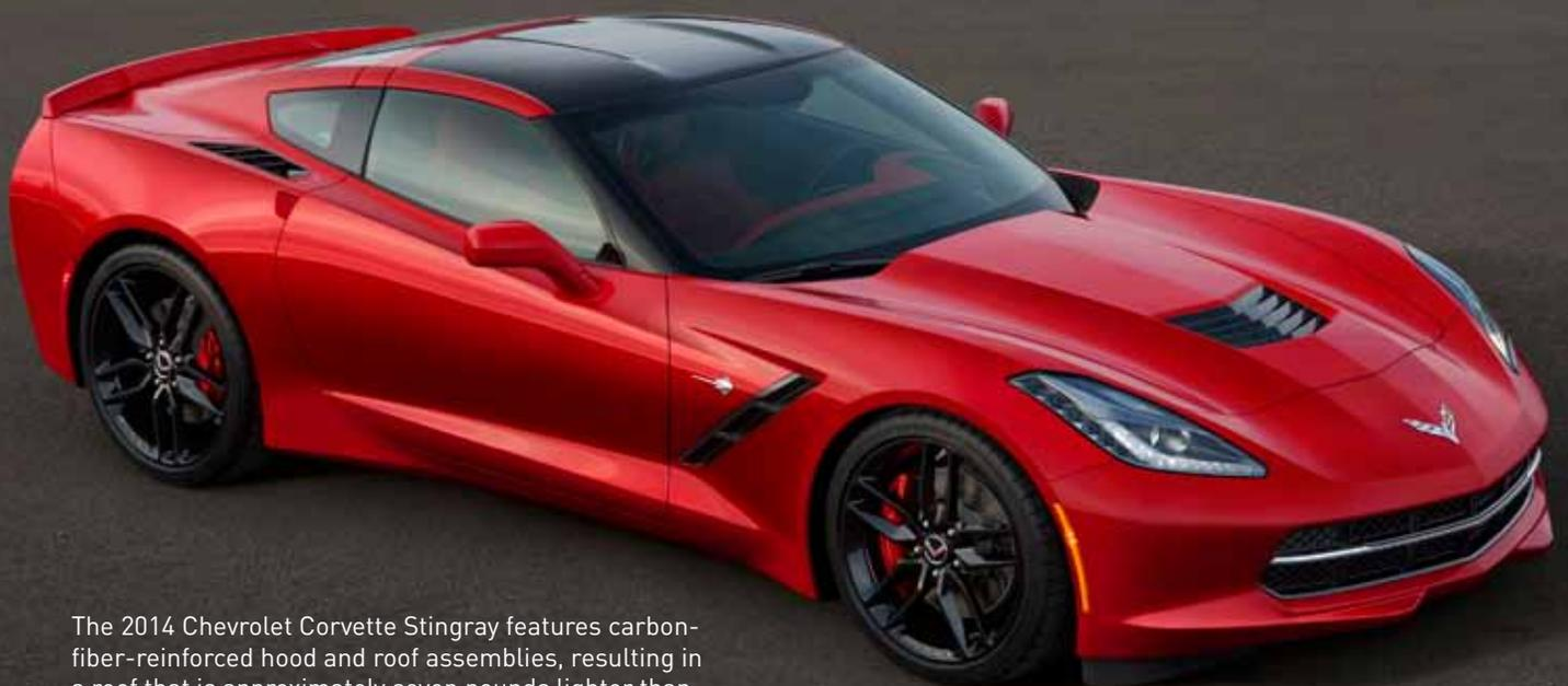
The 2014 Chevrolet Corvette Stingray features carbon-fiber-reinforced hood and roof assemblies, resulting in a roof that is approximately seven pounds lighter than the previous version. In addition, panel gap consistency was improved by 30% and part costs/unit area were reduced roughly 40% compared to the previous model.
