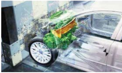
Energy absorption of a front crumple zone
